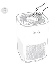
After switching on the power, press and hold the filter replacement button for 3 seconds, and when you hear the beep, the installation is successful.
