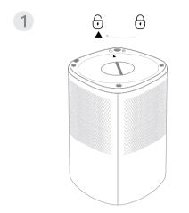
Placing the machine bottom up, rotate the bottom cover counterclockwise to unlock it
